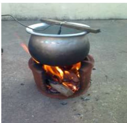
Fig. 2 Biomass stove without porous medium
